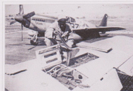
99th Fighter Squadron mechanic reloading a P-51 Mustang, during World War II.
